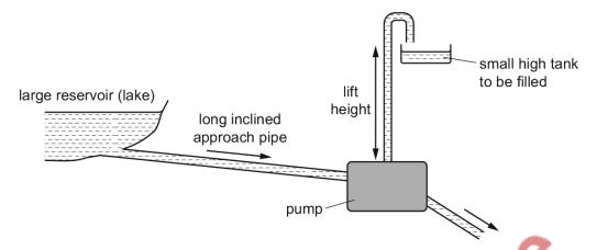
In one such pump the long approach pipe holds 500 kg of water. A valve shuts when the speed of this water reaches 2.0 m s<sup>-1</sup> and the kinetic energy of this water is used to lift a small quantity of water by a height of 15 m.
